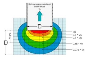
Figure 2: Suction field on the hood as a function of the flow velocity and Inlet diameter (in accordance with DGUV rule 109-002, p.15).
