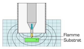
Figure 1Plasma nozzle and substrate position in the suction field
